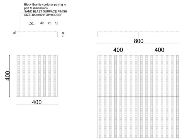
CORDUROY PAVING HAZARD WARNING PAVING FOR BOTTOM AND TOP OF STEPS
